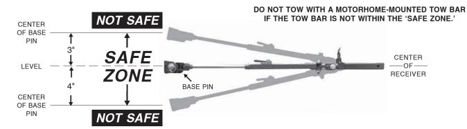
Towing with a motorhome-mounted tow bar which has an upward or downward slope puts undue strain on the entire towing system. DO NOT TOW if the tow bar is not within the 'Safe Zone' – no more than 3 inches above level or 4 inches below level. Towing a vehicle with a tow bar that is not within the Safe Zone will result in significant wear and tear on the tow bar and brackets, significant wear and tear on the vehicle's suspension and frame, and the eventual failure of your towing system.
