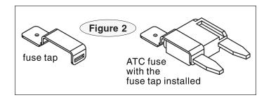
the 20-amp fuse and holder assembly must be installed within a few inches of the electrical connection. If the 20-amp fuse is farther than a few inches, a short circuit may cause an electrical fire, causing severe damage to the vehicle.
