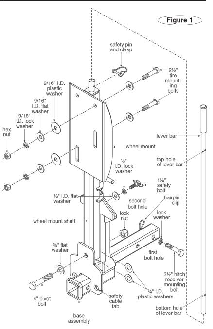
**2.** Although not required, we recommend using Loctite<sup>®</sup> Red on the 3½" hitch receiver mounting bolt.
