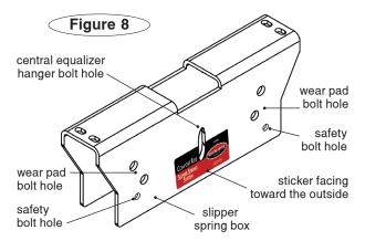
**d.** Position a 9/16" flat washer over one of the included 9/16" x 4" bolts and insert it through the central hole in the slipper spring box and the 2" pipe spacer. On the opposite side of the slipper spring box, finish with another 9/16" flat washer and 9/16" nylock nut. Leave loose at this time.
