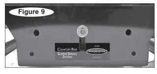
**9.** Align the slipper spring box so that it is in line with the trailer's frame rail and centered underneath the frame rail.
