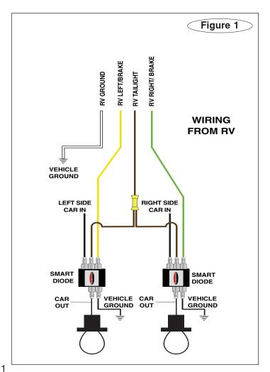
4. Now crimp the 12" white wire to the terminal labeled Ground and repeat for the other diode. Use the included ring terminals and Tek screws to ground both wires to the chassis.
