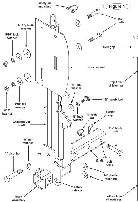
2. Although not required, we recommend using Loctite® Red on the 3½" hitch bolt.
