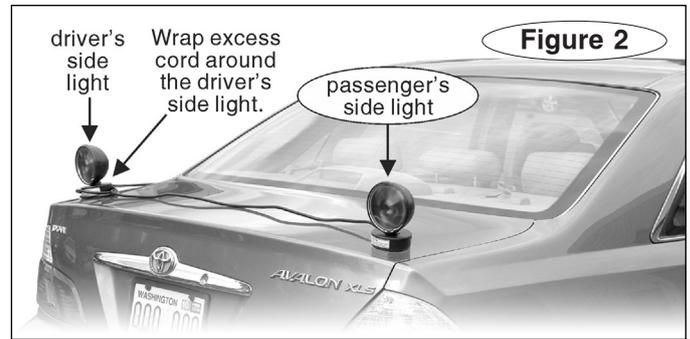
age to the towed vehicle's finish, make certain that both the underside of the magnets and the surface of the towed vehicle are clean.
