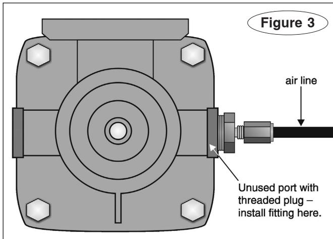
If an incorrect port is chosen, the motorhome brake system will be severely damaged. A brake fire or other non-warranty damage may also occur.
