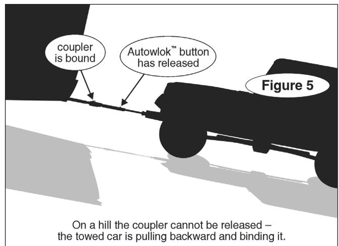
On a hill the coupler cannot be released – the towed car is pulling backward and binding it.
