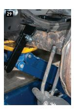
27) Original U-bolts will need to be closed slightly to fit in the new tie plates. This can be done by placing the nuts on the ends and hitting with a hammer while on a solid surface. 28) A vice can also be used to close the gap. 29) U-bolts are positioned under the axle and through the new tie plate, which is also the mounting bracket for the shock absorbers.
