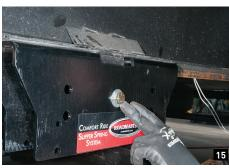
the system is brilliant when applied to trailer suspensions. It solves an inherent design problem, whereby leaf springs are tied to equalizer shackles and frame-mounted hangers via eyes in the spring ends, restricting the movement needed to smooth out the ride effectively.
