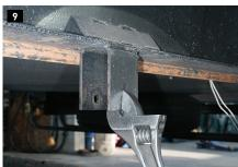
4) The U-bolt is removed and set aside for use later in the install. 5 and 6) The bolt is removed from each hanger and existing equalizer (7) so that the spring assembly (8) can be dropped from the frame. 9) Spring-hanger flanges will need to be spread slightly to make room for the new spring eyes. This can be done easily with an adjustable wrench. It's important not to open the spacing too wide.
