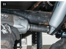
30) Once all the bolts are in place and snugged evenly, a torque wrench is used for final tightening. 31) Redlands Truck and RV Performance Center prefers to use torque paint to let other mechanics know that the bolts have been tightened to specified values. 32) Shock absorbers bolt to the center box using a wedge to keep them at the proper angle. 33) Once both ends are bolted and tightened properly, the retaining strap can be cut, allowing the shocks to seat into the mounting brackets.
