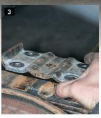
1) Jack stands are needed to support the frame and allow the suspension to hang. The trailer must not be lifted by the axles, which are stabilized only with floor jacks. 2 and 3) Once the tires are removed, the tie plates are unbolted to free the axles from the springs.
