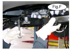
4. Hold a receiver brace under the subframe as shown (Fig.F) and bolt through the rear mounting hole with a 14mm x 2.0 x 140mm bolt, lock washer and flat washer.
