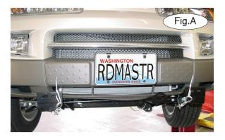
**IMPORTANT:** All baseplates **must** be assembled with all the bolts left loose for final adjustment and positioning (before tightening) unless otherwise instructed. All bolts **must** be torqued for proper strength. If more than one bolt is used per fastening point, the diagram may only show one. Use flat washers over all slotted holes and lock washers on all fasteners.
