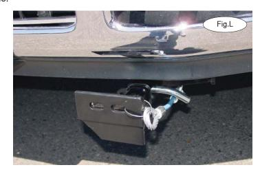
11. Attach the ends of the safety cables to the tow vehicle's safety cables and tow bar.
