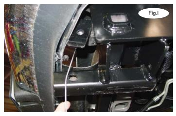
4. Place the  $\frac{1}{2}$ " x  $\frac{3}{2}$ " backing plate with weld nut and attached wire inside the frame (Fig.I). Bolt through the third hole back and into the backing plate with the weld nut, using the  $\frac{1}{2}$ " x  $\frac{1}{4}$ " bolt and lock washer. Repeat for the second hole back (Fig.J).
