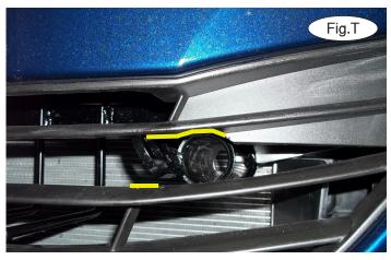
16. Hold the fascia in place over the receivers and mark it for trimming. Due to manufacturing variances, the grille will be one of the four patterns shown in Figures S, T, U or V. Match the pattern shown with the vehicle and trim using the yellow lines in the images as a guide to allow clearance for the main receiver brace.
