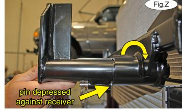
22. On each side, insert the removable front bracket arm into the front receiver 90 degrees from its final towing position, depressing the spring-loaded pin against the receiver (Fig.Y). Now, twist back 90 degrees until the spring-loaded pin snaps into place in the notch on the receiver, locking the arm into place in its final towing position (Fig.Z).
