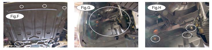
4. Remove the center splash shield by removing five 8mm (head) bolts, two plastic fasteners and two 10mm (head) bolts. The 8mm (head) bolts are in the front. The plastic fasteners and the 10mm bolts are in the rear of the splash shield. Next, remove two more 10mm (head) bolts per side, and one plastic fastener (Fig.F,G).
