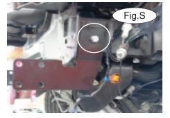
15. On both sides, bolt the side brace into place using two  $\frac{1}{2}$ " x  $1\frac{1}{2}$ " bolts and lock washers. Bolt through the existing holes in the frame rail (Fig.Q).
