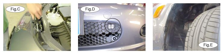
1. *Important:* please use all supplied bolts and parts and read all instructions carefully before beginning this installation. The majority of questions you may have can be answered within the text, and proper installation will ensure safe and secure travel. Now, begin the installation. Start by removing eight 10mm (head) bolts attaching the fascia to the core support (Fig.C). *Note:* due to manufacturing variances, newer models may have a different number of fasteners.
