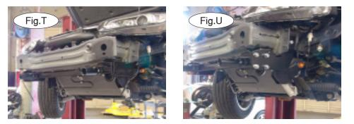
18. Now, bolt the bumper core back into place (Fig.T), reversing step 10.
