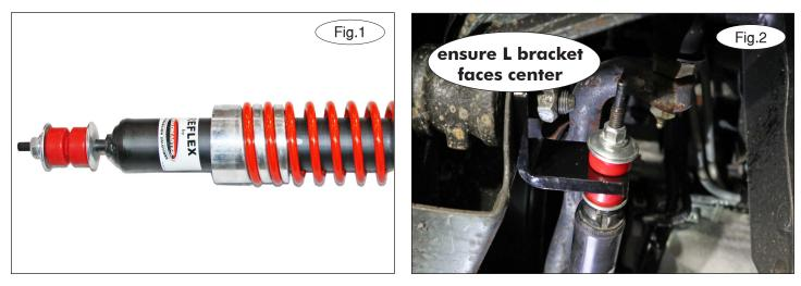
Note: Before installing the shock component of this system, please ensure that the spring is fullyseated in its track on the collar of the unit. If it is installed without the spring fully-seated in its track, the unit could malfunction or otherwise fail to operate properly (Fig.1).
