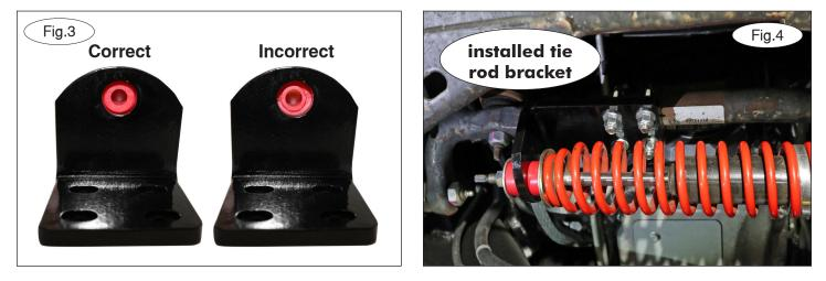
3. Loosely install the stabilizer to the chassis bracket. The end without the spring will attach to the chassis bracket. *Note: Ensure the bushings are oriented in the tie rod bracket hole as shown in Figure 3. Proper orientation of the bushing will keep the Reflex unit centered in the bracket. Note that the bracket shown in Figure 3 may vary by kit.*
