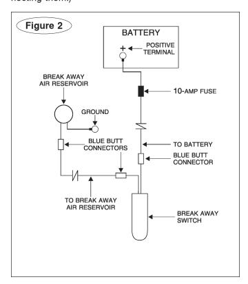
Next, route the wire to the positive terminal on the towed vehicle's battery (Figure 2), avoiding moving parts, sharp edges or "hot" components such as the engine or exhaust system. Where appropriate, use one or more of the included wire ties to secure the wire in place.
