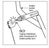
**4.** Make certain that no part of the brake pedal clamp, and/or the two Allen head bolts, will interfere with the driver's foot or the normal operation of the vehicle. If they will, trim them.
