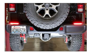
strip is flexible. Use care to make certain that the light strip is mounted straight. Once properly positioned, press firmly on the LED strip for maximum adhesion (Figure 1).
