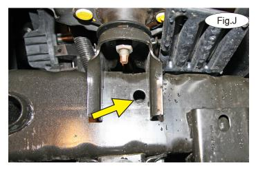
4. Starting on the passenger side, locate the existing hole on the inside and outside of the frame rail (Fig.J – outside). *Note:* due to manufacturing variances, the hole in the outside of the frame rail may not exist. If this is the case, use a  $\frac{1}{2}$ " drill bit to drill straight through the inside hole.
