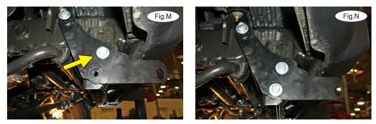
6. Bolt through the uppermost hole, the main receiver brace and side-specific brace using the supplied  $\frac{1}{2}$ " x 1<sup>3</sup>/<sub>4</sub>" bolt,  $\frac{1}{2}$ " flat washer and  $\frac{1}{2}$ " lock washer. Place a 1<sup>1</sup>/<sub>2</sub>" x 3" nutted backing plate in the frame and over the bolt (Fig.M).
