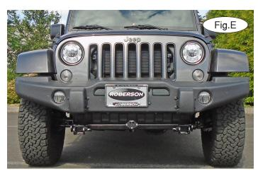
If you have a Winter Edition model or any other model with a bumper like the one shown in Figure E: trim the skid plate as shown in Figure F. *Note:* before moving onto step 2, check that the threaded backing plate can easily fit into the end of the subframe (Fig.G). If it can't, trim the skid plate until it can.
