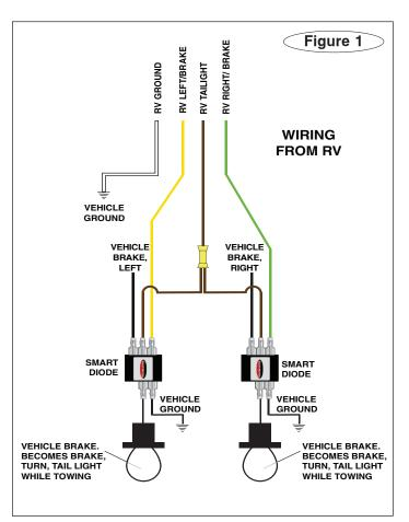
**5.** Now crimp the 12" white wire to the terminal labeled Ground and repeat for the other diode. Use the included ring terminals and Tek screws to ground both wires to the chassis.
