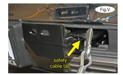
*Note:* if the bracket is so equipped, the holes in the alignment tabs which are welded to the arms and main receivers are for padlocks only. Under no circumstances should you bolt the alignment tabs together. Bolting the alignment tabs together may result in non-warranty damage to the bracket.
