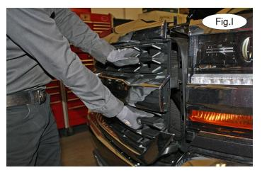
6. For 2015 and earlier models: skip to step 7. For 2016 and later models: on each side, pull up on the corner of the upper grille to pull the aligning pin out of the slot (Fig.H). Ensuring that the pin is properly released, get a firm grip on the side of the fascia and pull straight out on it to release the clips from the side and bottom of the upper grille (Fig.I). Now, skip to step 8.
