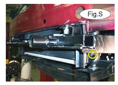
18. Tighten the front and rear bolts to the bolt torque requirements found at the end of this document.
