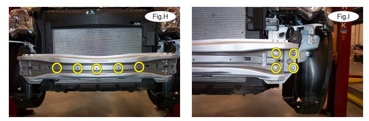
6. Unsnap five plastic clips to remove the wiring harness from the back of the bumper core (Fig.H).
