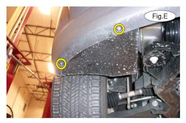
3. On each side, remove two 7mm (head) bolts attaching the bottom of the fascia to the fender liners (Fig.E).
