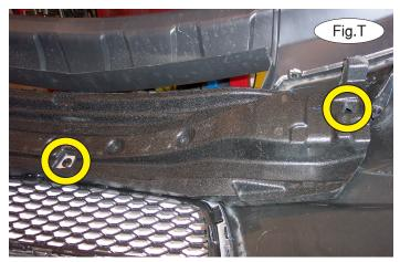
20. Remove the foam shock absorption pad from the back of the fascia by removing two plastic clips and one screw. Figure T only shows one clip and the screw. *Note:* due to manufacturing variances, some vehicles may have four clips.
