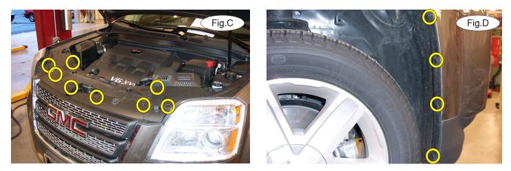
1. Important: please use all supplied bolts and parts and read all instructions carefully before beginning this installation. The majority of questions you may have can be answered within the text, and proper installation will ensure safe and secure travel. Now, begin the installation by removing four plastic fasteners and four T20 Torx bolts attaching the top of the fascia to the core support (Fig.C).
