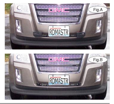
**IMPORTANT:** All baseplates **must** be assembled with all the bolts left loose for final adjustment and positioning (before tightening) unless otherwise instructed. All bolts **must** be torqued for proper strength. If more than one bolt is used per fastening point, the diagram may only show one. Use flat washers over all slotted holes and lock washers on all fasteners.
