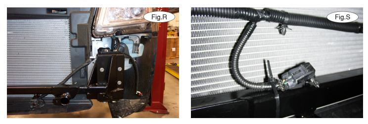
17. Bolt the upper brace into place using one of the supplied ½" x 1½" bolts, lock washers and nuts (Fig.R).
