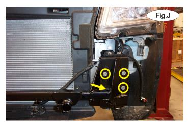
8. Place thread lock on six of the eight bolts you removed in the previous step and use them to attach the main receiver brace to the ends of the frame rails (Fig.J). Note: due to manufacturing variances, one of the mounting holes may be where the yellow arrow is instead. Tighten the bolts to the bolt torgue requirements found at the end of these instructions.
