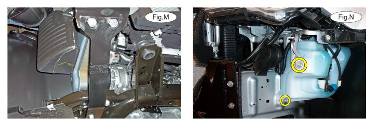
11. Using two of the supplied 1/2" x 11/4" bolts, lock washers and nuts, bolt the lower brace to the main receiver brace (Fig.M). Tighten the bolts to the bolt torque requirements found at the end of this document.
