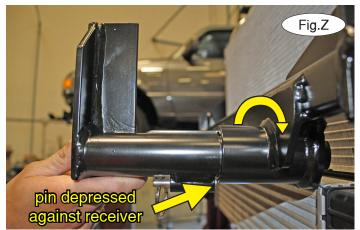
26. On each side, insert the removable front bracket arm into the front receiver 90 degrees from its final towing position, depressing the spring-loaded pin against the receiver (Fig.Z). Now, twist back 90 degrees until the spring-loaded pin snaps into place in the notch on the receiver, locking the arm into place in its final towing position (Fig.AA).
