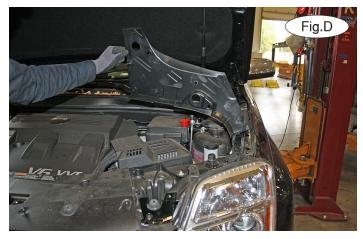
1. *Important:* please use all supplied bolts and parts and read all instructions carefully before beginning this installation. The majority of questions you may have can be answered within the text, and proper installation will ensure safe and secure travel. Now, begin the installation. On each side, remove three plastic fasteners attaching the engine cover to the top of the fascia (Fig.C). Fold it back out of the way (Fig.D).
