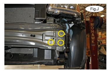
7. On each side, remove three 13mm (head) bolts attaching the bumper core to the frame rails (Fig.J). The bumper core will not be replaced. Retain the bumper core in case the bracket is ever removed.
