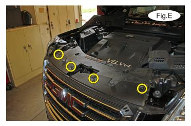
2. Remove four T20 Torx screws attaching the top of the fascia to the core support (Fig.E).
