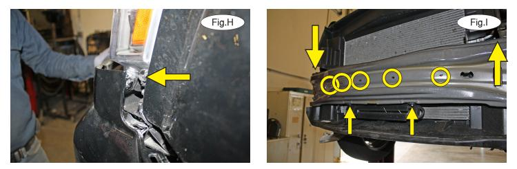
5. Pull out on the corners of the fascia to remove it. Note: if the corners are not easily removed, you may need a pry tool to release the corners at the spot indicated with an arrow in Figure H.
