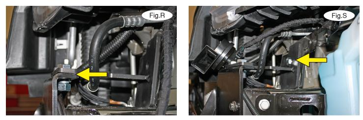
16. Working on the driver's side only, maneuver the upper mounting brace around the wiring harness and cooling line and over the top of the main receiver brace. Using two of the supplied  $\frac{1}{2}$ " x 1<sup>1</sup>/<sub>4</sub>" bolts, lock washers and nuts, bolt the upper mounting brace to the main receiver brace (Fig.R).
