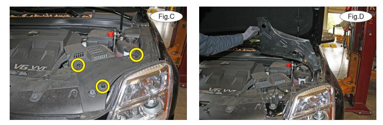
1. *Important:* please use all supplied bolts and parts and read all instructions carefully before beginning this installation. The majority of questions you may have can be answered within the text, and proper installation will ensure safe and secure travel. Now, begin the installation. On each side, remove three plastic fasteners attaching the engine cover to the top of the fascia (Fig.C). Fold it back out of the way (Fig.D).
