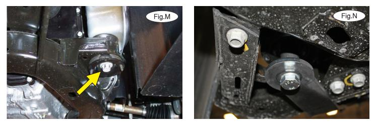
10. Working on the driver's side only, remove the 18mm subframe bolt. *Note:* do not remove both subframe bolts without supporting the frame (Fig.M). *Note:* due to manufacturing variances, there may be additional framing present that is not represented in Figure M.
