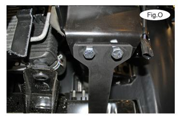
12. Using two of the supplied  $\frac{1}{2}$ " x 1<sup>1</sup>/<sub>4</sub>" bolts, lock washers and nuts, bolt the lower rear brace to the main receiver brace (Fig.O). Tighten the bolts to the bolt torque requirements found at the end of this document. *Note:* use Loctite® Red on all nuts and bolts.
