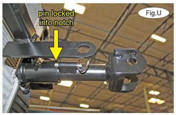
18. On each side, insert the removable front bracket arm into the front receiver 90 degrees from its final towing position, depressing the spring-loaded pin against the receiver (Fig.T). Now, twist back 90 degrees until the spring-loaded pin snaps into place in the notch on the receiver, locking the arm into place in its final towing position (Fig.U).
