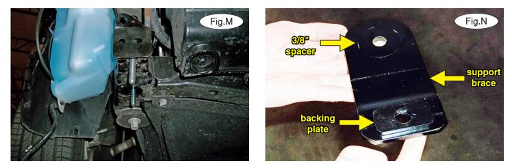
11. On each side, using one of the supplied  $\frac{1}{2}$ " x  $1\frac{1}{2}$ " bolts, bolt down through the pre-existing hole in the top of the sub-frame and through the backing plate you installed in the previous step (Fig.M – passenger side).
