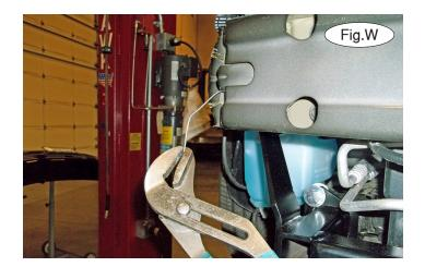
19. On each side, use a pair of channel locks to bend the rod on the backing plate out of the way (Fig.W).
