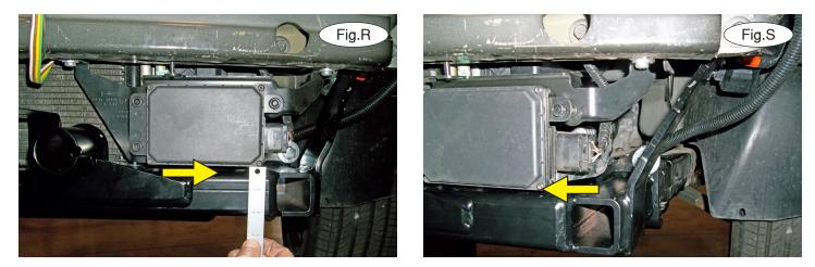
14. Measure to make certain that the ACC unit is properly spaced from the main receiver brace so there isn't any contact between them. There should be approximately ¼" of space between the bottom of the ACC unit and the main receiver (Fig.R). *Note:* ensure the bracket is properly aligned before proceeding to the next step (Fig.S).
