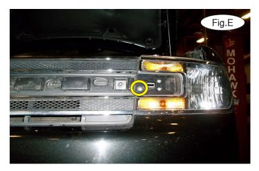
3. On each side, remove one 10mm (head) bolt attaching the upper grille to the core support (Fig.E).
