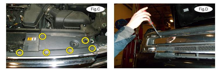
1. *Important:* please use all supplied bolts and parts and read all instructions carefully before beginning this installation. The majority of questions you may have can be answered within the text, and proper installation will ensure safe and secure travel. Now, begin the installation. On each side, remove four 5.5mm (head) screws, one 10mm bolt and one plastic fastener attaching the radiator cover to the core support (Fig.C – driver's side).
