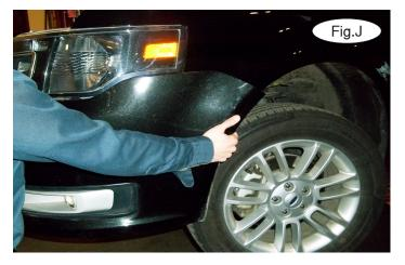
8. Pull out and forward on the corners of the fascia to remove it from the locking strip on each side (Fig.J). Disconnect the fog lights, if the vehicle is so equipped.
