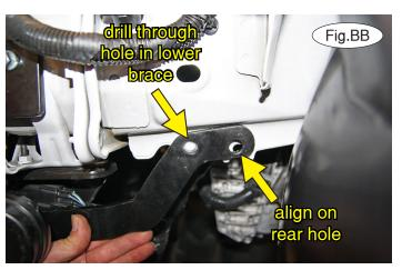
23. On the driver's side only, locate the slip nut on the pinch weld computer mount and remove it (Fig.AA). Then, take the lower brace and bolt it to the side brace as in step 22 using a  $\frac{1}{2}$ " x 2" bolt. Finish with a  $\frac{1}{2}$ " lock washer and  $\frac{1}{2}$ " nut. Now, hold the lower brace firmly against the pinch weld and mark the forward hole and drill (Fig.BB). *Note:* the rear hole of the lower brace should align roughly with the computer mount.
