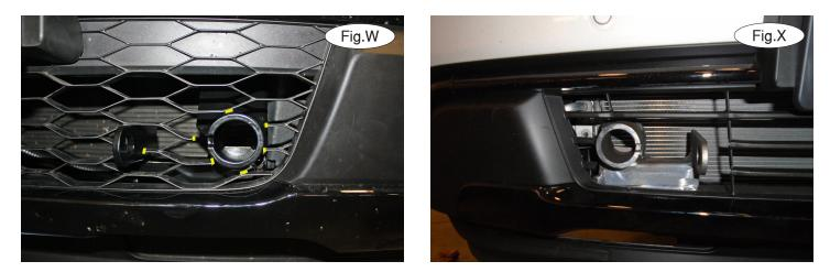
19. Hold the fascia over the main receiver brace and trim as necessary to allow clearance around the receiver and safety cable tab. For '16-'17 models: trim as shown in Figure W. For '18 and later models: trim as shown in Figure X. *Note:* trimming may also be needed to allow clearance around the wiring plug mounts.
