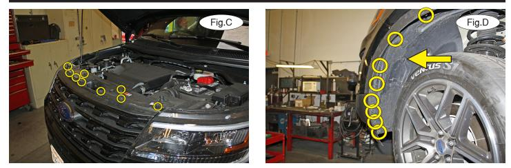
1. *Important:* please use all supplied bolts and parts and read all instructions carefully before beginning this installation. The majority of questions you may have can be answered within the text, and proper installation will ensure safe and secure travel. Now, begin the installation by removing seven 10mm (head) bolts and two plastic fasteners attaching the radiator cover to the core support (Fig.C).
