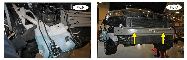
10. On the passenger side, remove one 8mm (head) bolt and two 11mm (socket) nuts attaching the washer bottle to the frame and then maneuver the washer bottle neck carefully out of the frame (Fig.N) and secure the washer bottle away from the frame for now. *Note:* if the washer bottle has a wiring harness attached to a cooling line, unplug it.
