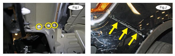
6. On each side, pull out the fender liner far enough to gain access to three 10mm (head) bolts attaching the fascia to the fender (Fig.I – passenger side). Remove them.
