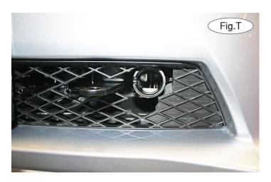
17. Trim the fascia as shown in Figure T to allow clearance for the main receiver brace.
