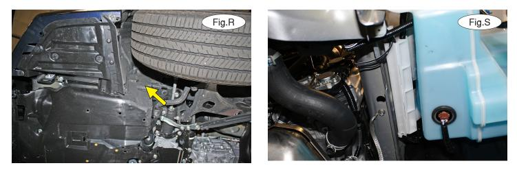
14. On each side, place a  $\frac{1}{2}$ " clipped plate washer over one of the supplied  $\frac{1}{2}$ " x 5" bolts and bolt through the back of the frame and out the front lower mounting point of the main receiver brace. Finish with a  $\frac{1}{2}$ " lock washer and nut (Fig.R and Fig.S).
