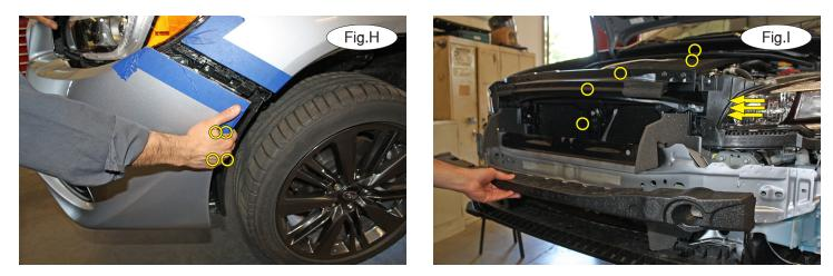
6. On each side, remove four 12mm (head) bolts attaching the bumper core to the frame rail (Fig.H – driver's side). It will not be replaced. *Note:* retain the bumper core and its attachment hardware so it can be replaced if the bracket is ever removed.
