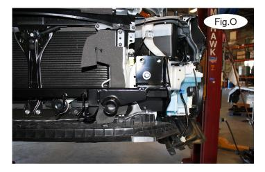
11. On each side, bolt the main receiver to the ends of the frame rails using the four supplied 8 mm x 1.25 x 35 mm bolts, 8 mm lock washers and  $5/16^{\circ}$  flat washers (Fig.O).
