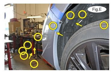
3. Remove nine plastic fasteners and four 10mm (head) screws attaching the bottom of the fender liner to the fascia and the splash shielding (Fig.E).
