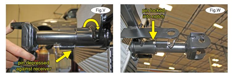
19. On each side, insert the removable front bracket arm into the front receiver 90 degrees from its final towing position, depressing the spring-loaded pin against the receiver (Fig.V). Now, twist back 90 degrees until the spring-loaded pin snaps into place in the notch on the receiver, locking the arm into place in its final towing position (Fig.W).
